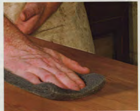
Steel wool is next. Available in rolls and pads, 0000 steel wool should be refolded to form a loose pad slightly larger than your hand.
