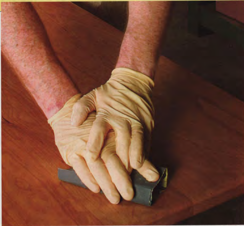
Flatten and dull the surface. Use 600-grit wet-or-dry sandpaper lubricated with mineral spirits to smooth the tabletop and remove any shiny low spots.
